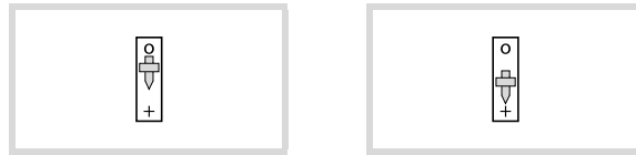
Switched off bus termination resistor
